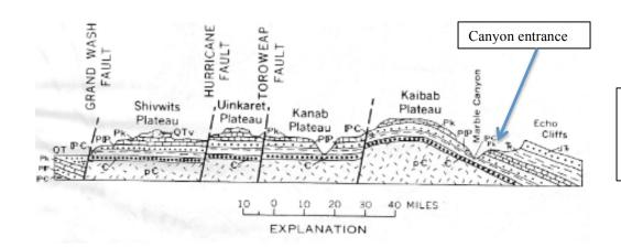
E-W Geologic section of northwestern Arizona; Shows the barrier to westward flow of the ancestral Colorado River<sup>1</sup>
